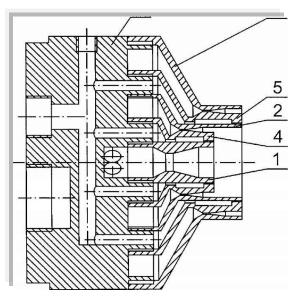
Magnetic cavitation nozzle for mixingatomic nitrogen with nanoparticles
